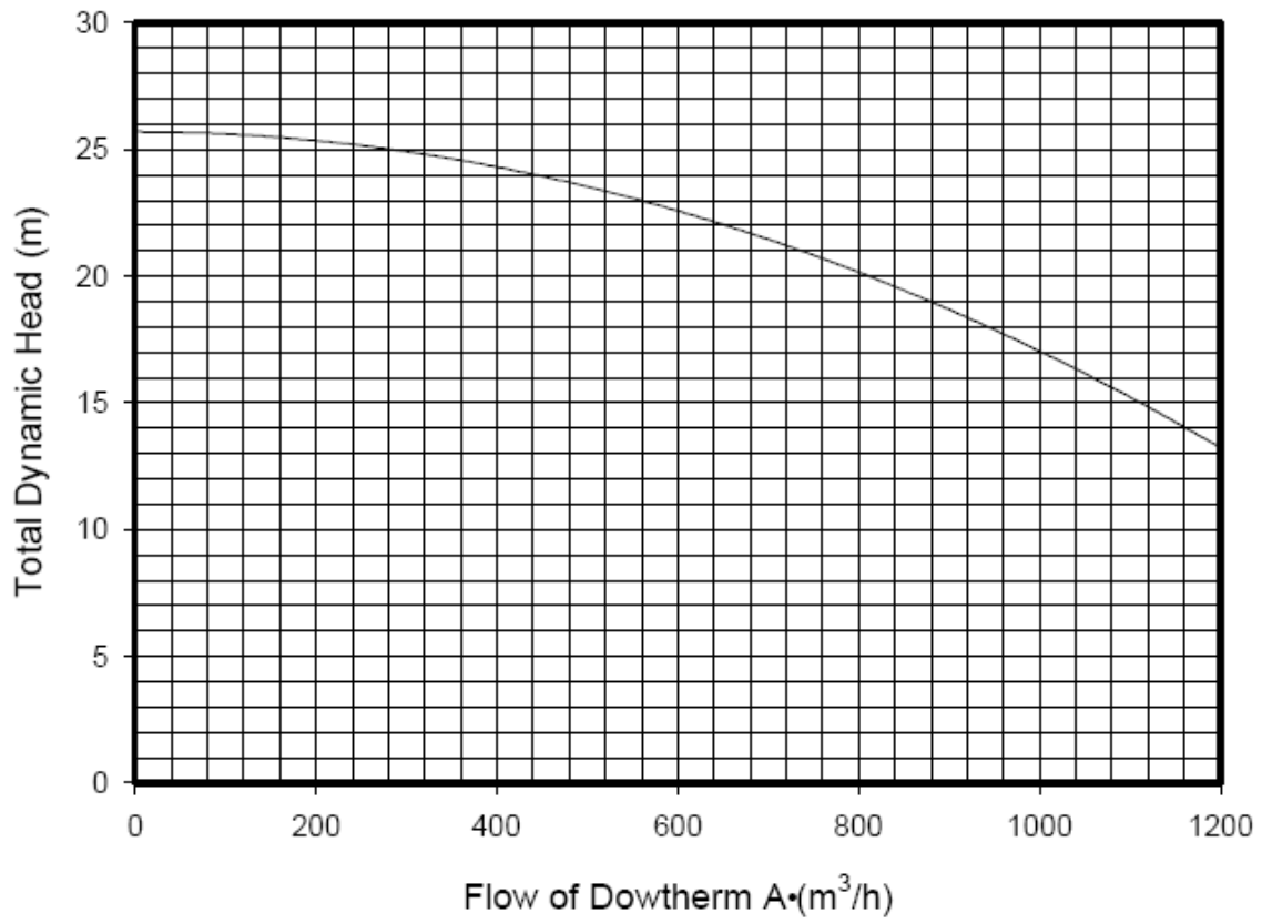
Pump Curve for the Dowtherm A Pump
