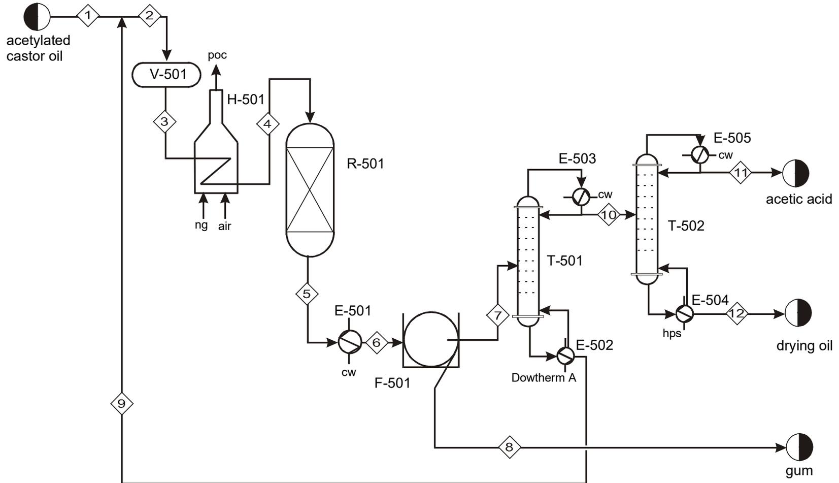
Figure 1: Preliminary Process Flowsheet for Drying Oil Production
