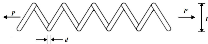
Figure 14. Schematic of the tension/compression spring design.
